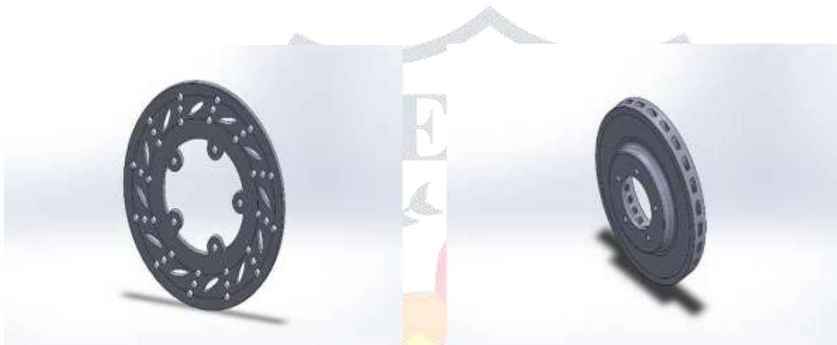
Figure.5 (a) Isometric view of drilled contour disc rotor. Figure.5 (b) Isometric view of ventilated disc rotor.
