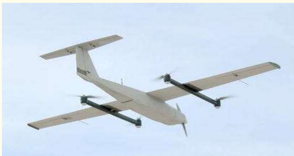
Figure 4. A hybrid fixed-wing-multi-rotor UAV
