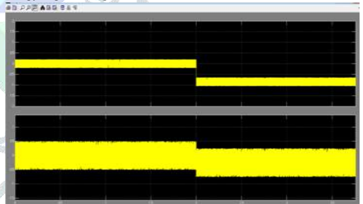
Fig.4.5. Waveforms of controlled current step change in the low-voltage dual-source-powering mode by simulation
