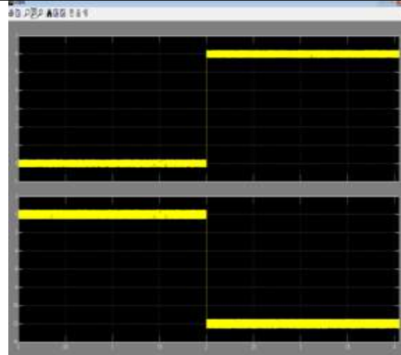
Fig. 4.9 Waveforms of controlled current step change in the low-voltage dual-source buck mode: by simulation
