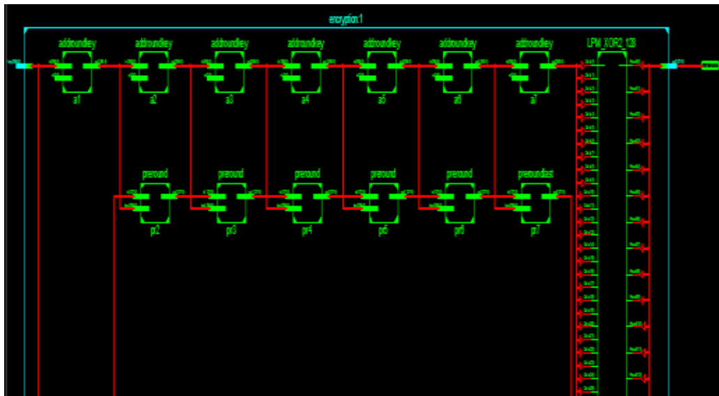
Figure 4: RTL view of proposed MAES algorithm
