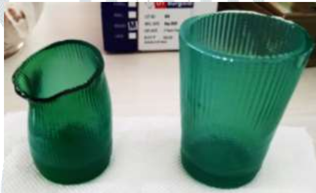
Figure 5. Deformation of Edible glasses when kept at 4°C for 10 days (left). Deformation of Edible glasses when kept at 4°C for 7 days (right).
