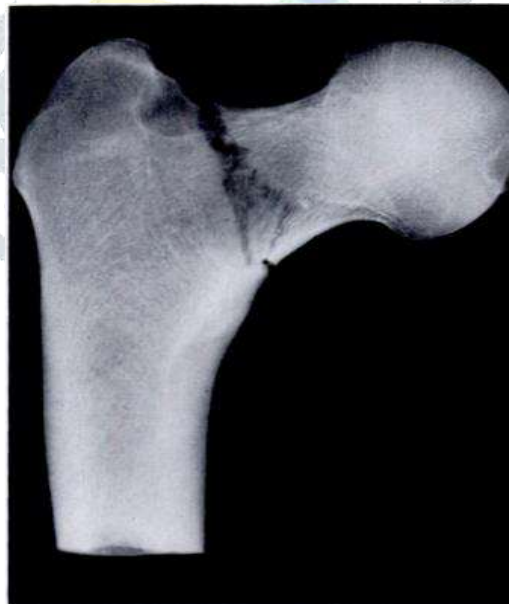
Fig.3 Fatigue failure at epiphysis head of Human bone [1]
