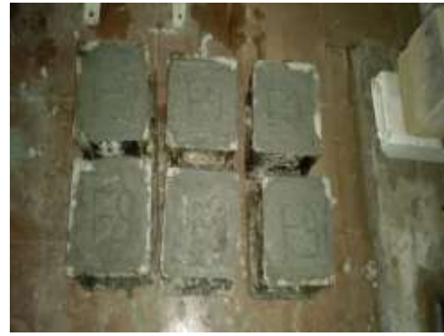
Fig 5: concrete block casting.
