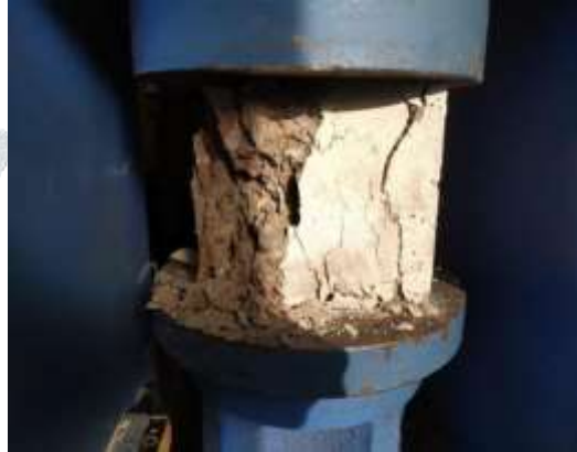
Fig 6. Failure of cube during strength testing in CPM.
