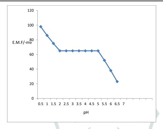
Fig: - Effect of pH on cell potential based electrodes No.2 [Pb<sup>2+</sup>] =1.0×10<sup>-3</sup> M
