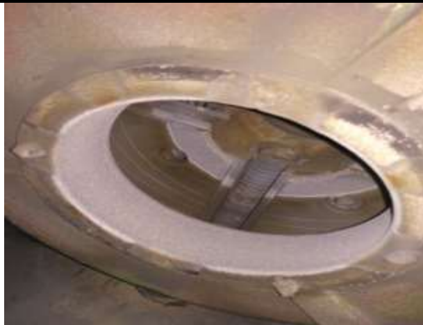
Figure 6.2 : Material coated bush on lathe
