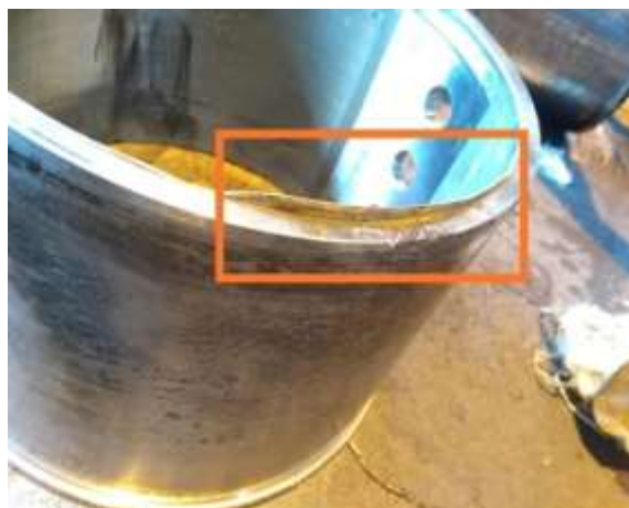
Figure 3.1 : wear out of the babbitt material
