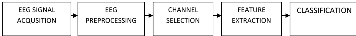
Fig. 1. Setup for EEG categorization with channel selector
