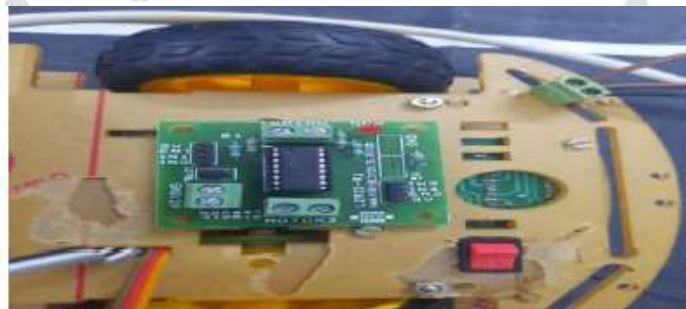
Fig. 4.2.2 L298N Motor Driver
