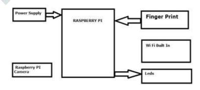
Figure 1. Work flow of Proposed System
