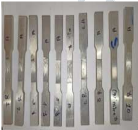
Fig 3.5: Tensile test specimen as per ASTM E8 standard
