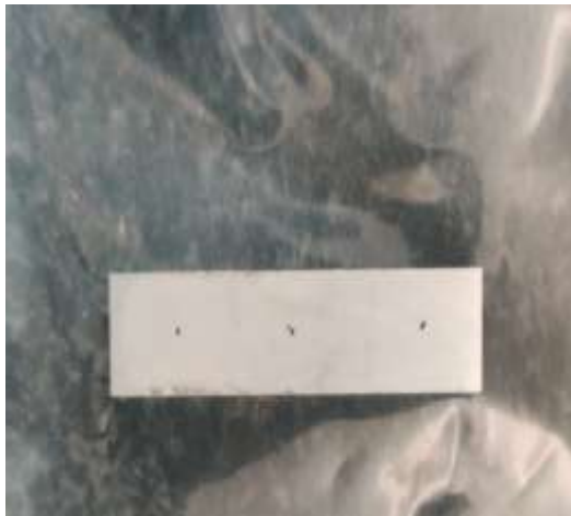
Fig 3.7: Polished hardness test specimen
