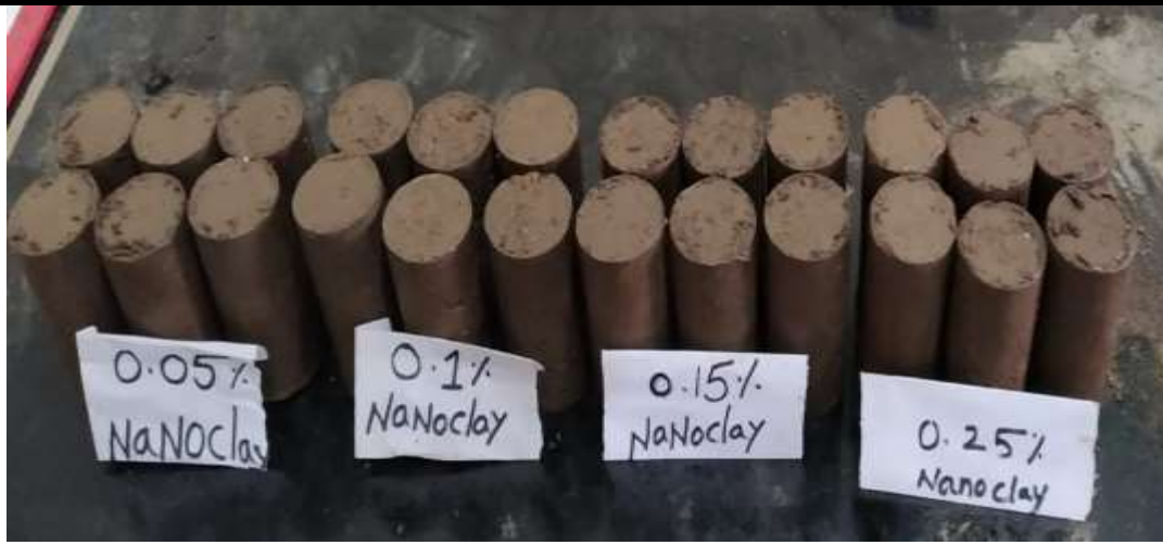
Fig. 5 Soil specimens for index and engineering properties
