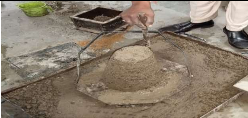
Fig. 1. Workability of concrete using slump cone method
