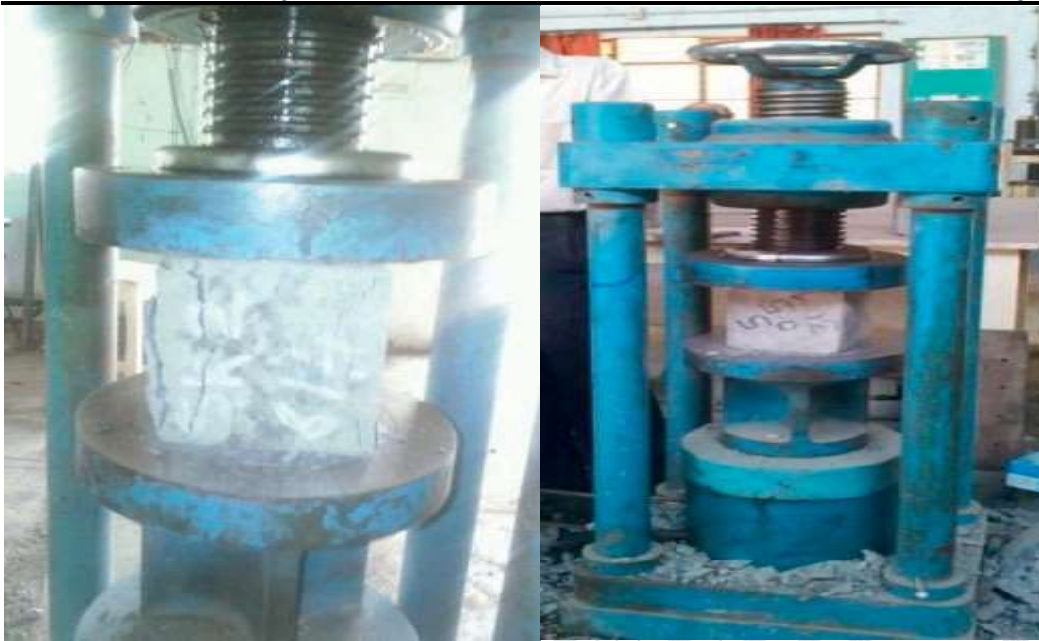
Fig 2: Testing of specimen under compression
