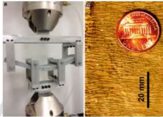
Figure 1.2. ECC has a high degree of deformability while also being resistant to brittle fracture. Under bending strain (a) and direct tension (b).
