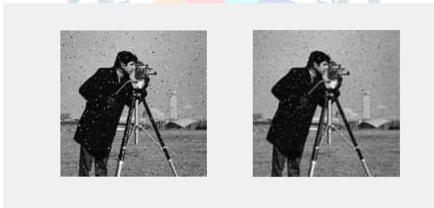
Fig 6.1 : (a) Noisy image (Salt and Pepper noise) (b) Ideal low pass filtered image
