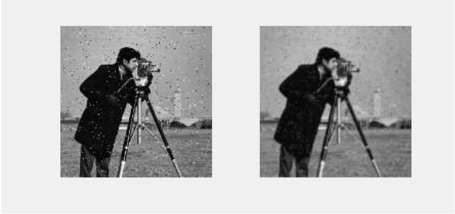
Fig 6.3:(a) Noisy image (Salt and Pepper noise) (b) Butterworth low pass filtered image
