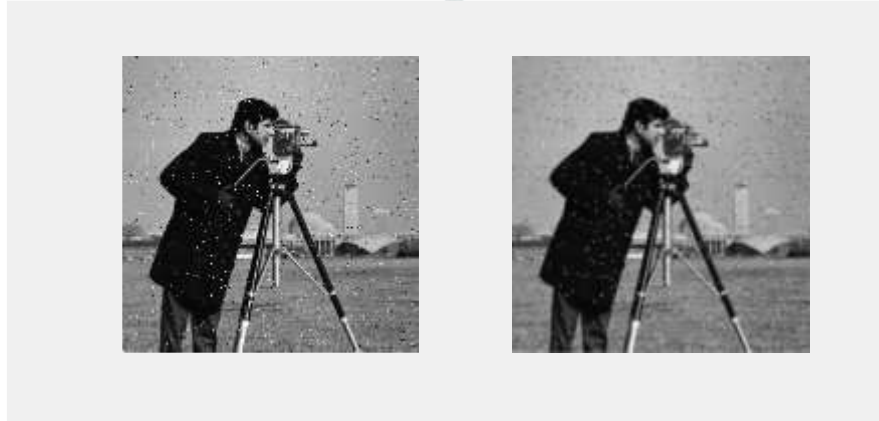
Fig 6.2: (a) Noisy image (Salt and Pepper noise) (b) Gaussian low pass filtered image
