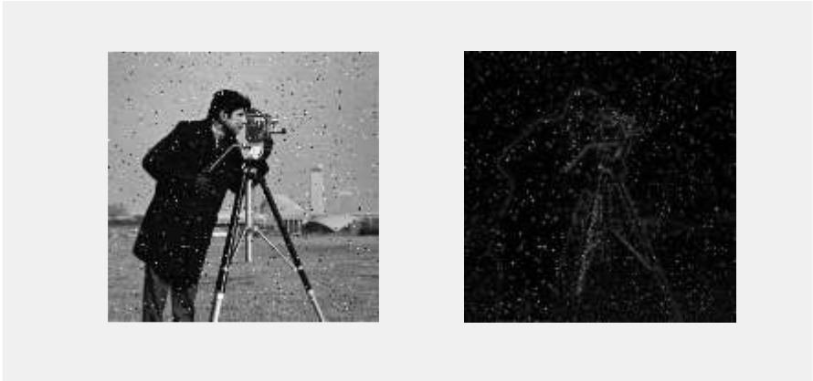
Fig 6.4:(a) Noisy image (Salt and Pepper noise) (b) Ideal high pass filtered image
