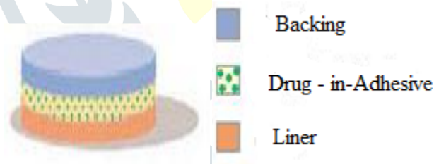
Fig.No. 2 Single-layer Drug-in-Adhesive
