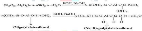
Figure 1.2 Geo-polymerization Reaction
