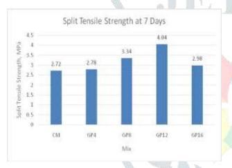
Figure 4. Split Tensile Strength Test Results at 7 Days.
