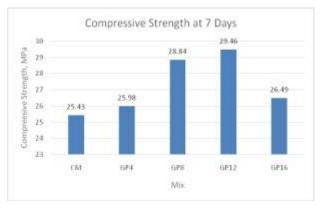
Figure 2. Compressive Strength Test Results at 7 Days.
