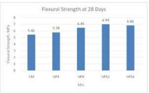
Figure 7. Flexural Strength Test Results at 28 Days.
