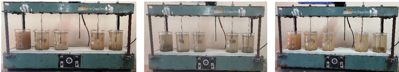
Fig. – 4 Optimization of dose of Dhavādi Bhasma by Jar test method
