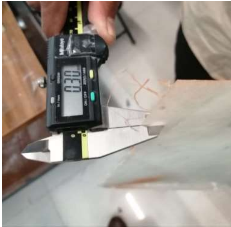
Fig 2 Thickness of Cured glass fiber (3 layers)
