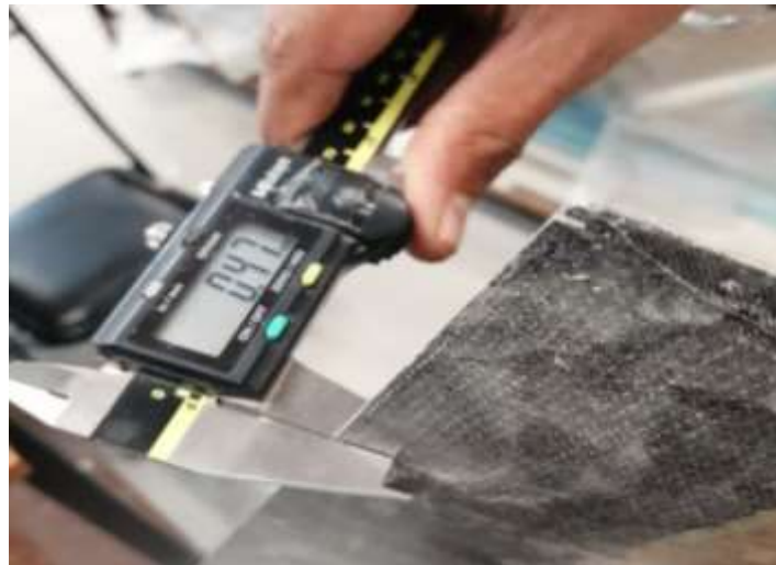
Fig 10 Thickness of Hybrid 1 (Carbon fiber + Glass fiber)
