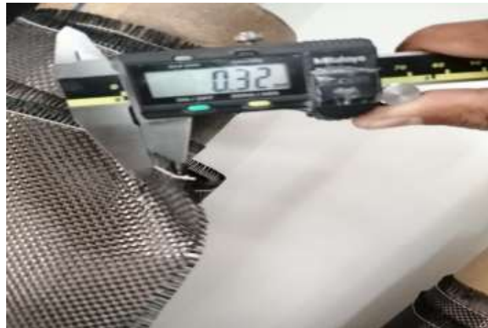
Fig 5 Thickness of carbon fiber 200 grams per square meter
