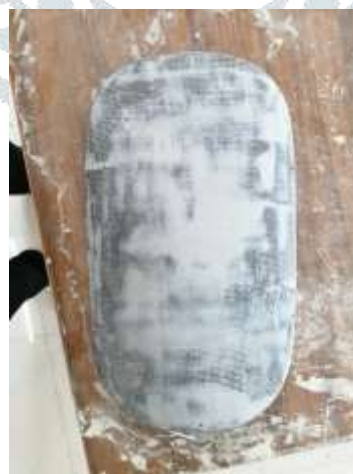
Fig 5 As the surface finish was not enough we need to add soft cut putty for the good finish
