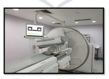
Figure 2. Symbia gamma camera from Siemens
