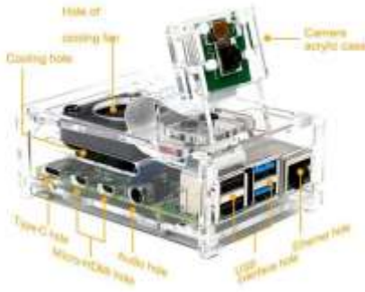
Fig3.3 Assembly of Raspberry pi 4B with camera
