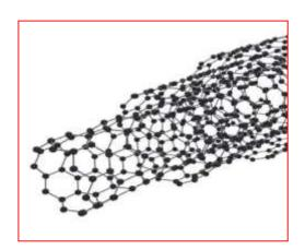
A) Single walled carbon nano tube
