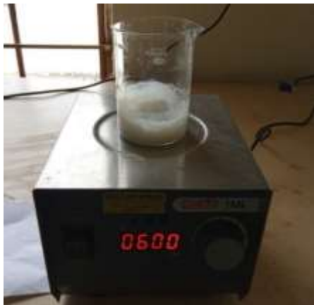
Figure 1: (a) The mixture of seed gel stirred at 600rpm (b) Seed gel formation
