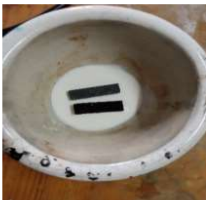
Figure 4: (a) Zeolite Na Y synthesis solution (b) Zeolite Na Y dried at 100°C (d) Graphite anodes dipped in Zeolite Na Y solution (e) Graphite anodes dried at 80°C.
