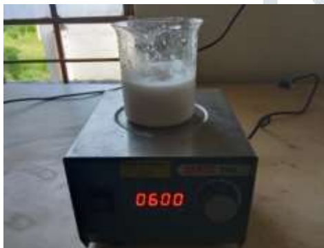
Figure 2: (a) The mixture of feedstock gel stirred at 600rpm (b) feedstock gel formation
