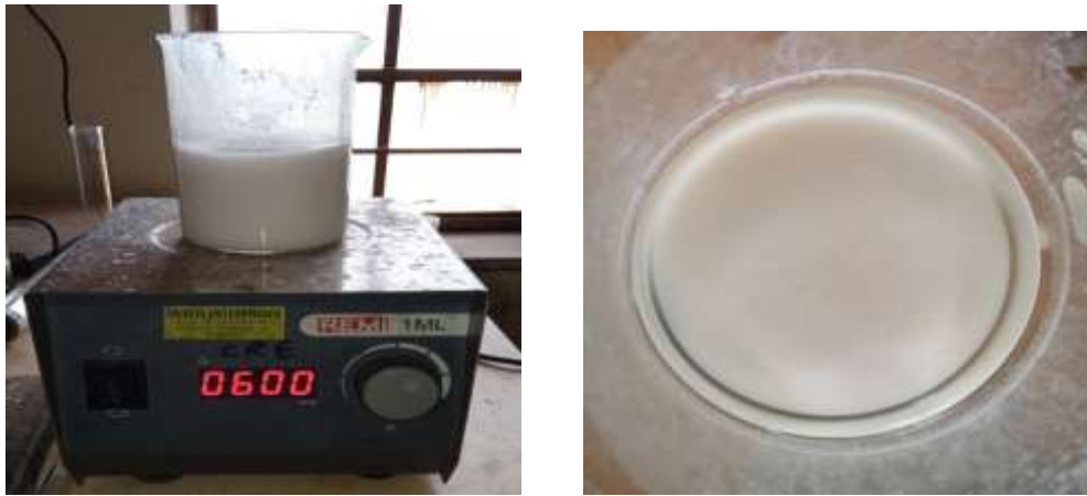
Figure 3: (a) The mixture of overall gel stirred at 600rpm (b) overall gel formation
