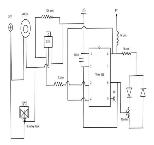
Figure 2 Circuit diagram of speed controller
