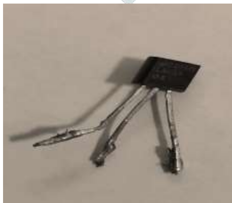
Figure 3 - LM35 Temperature Sensor
