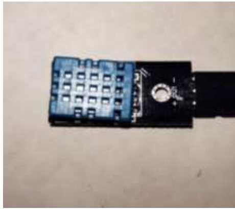
Figure 4 - Humidity And Temperature Sensor
