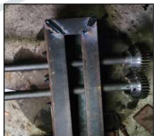
Fig 4.1 Fabrication of c-channel and shaft
