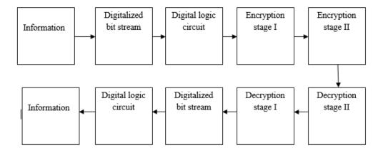
In this block diagram, information is the input image. The input image is then converted into the digitized bit stream. This bit stream is taken for the encryption and decryption stages. The resultant bit stream is then converted into the original image which is the input. Conversion of the image into bit stream and bit stream into an image is done by using the Matlab software.
