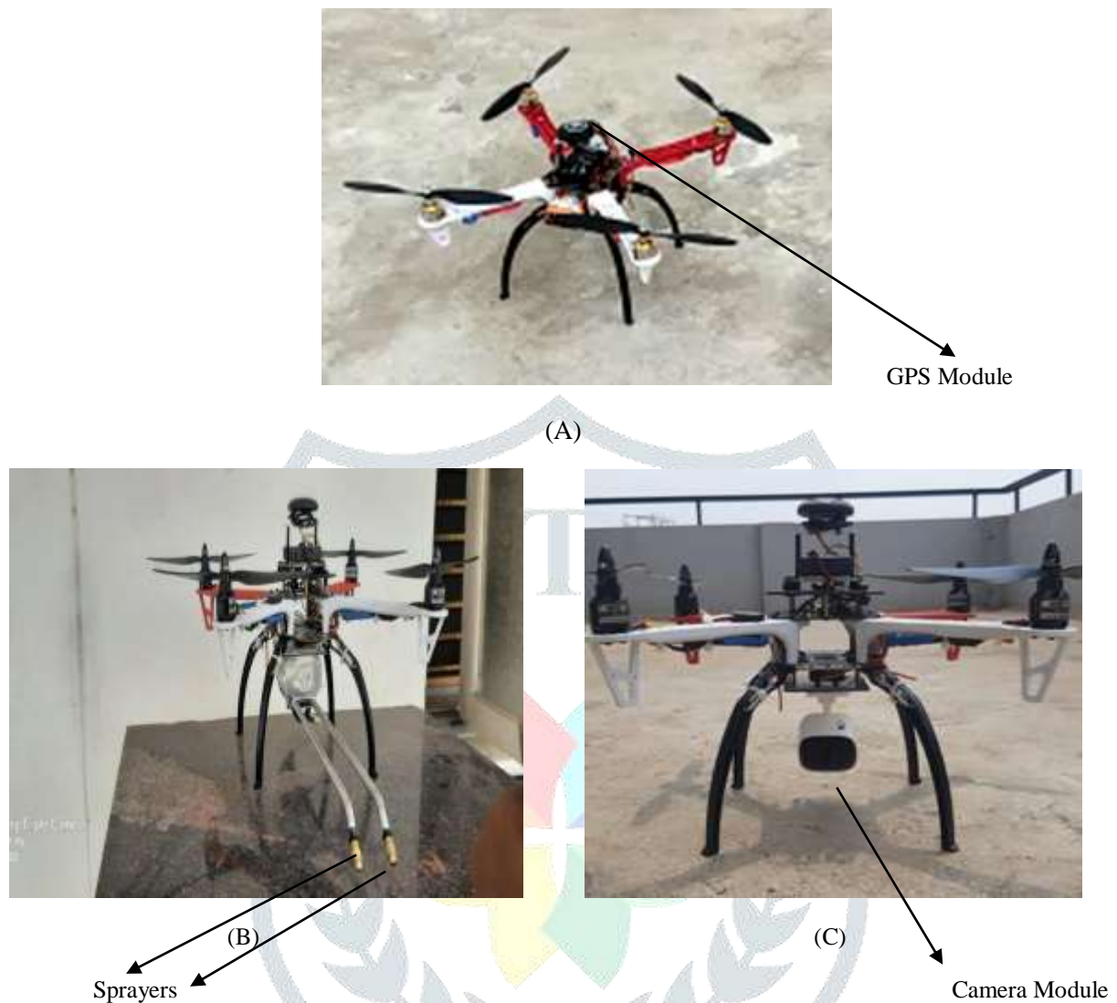
Fig. 7: (A) Drone with GPS Module, (B) Drone with Sanitization & (C) Drone with Surveillance Variants.
