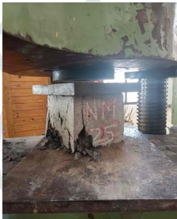
Fig.3 Compressive test on Cube
