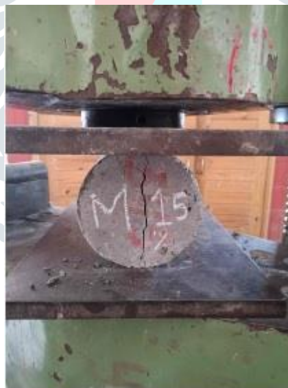
Fig.5 Split tensile test on Cylinder
