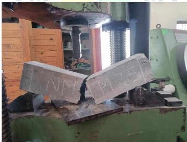
Fig.7 Flexural Strength Test on Beam
