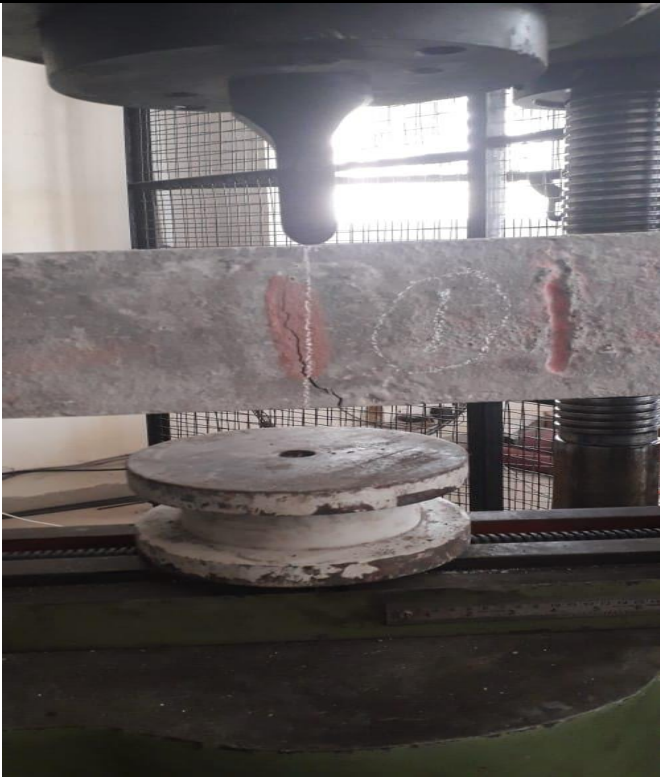
Fig. 1. Cracks developed in Conventional slabs.
