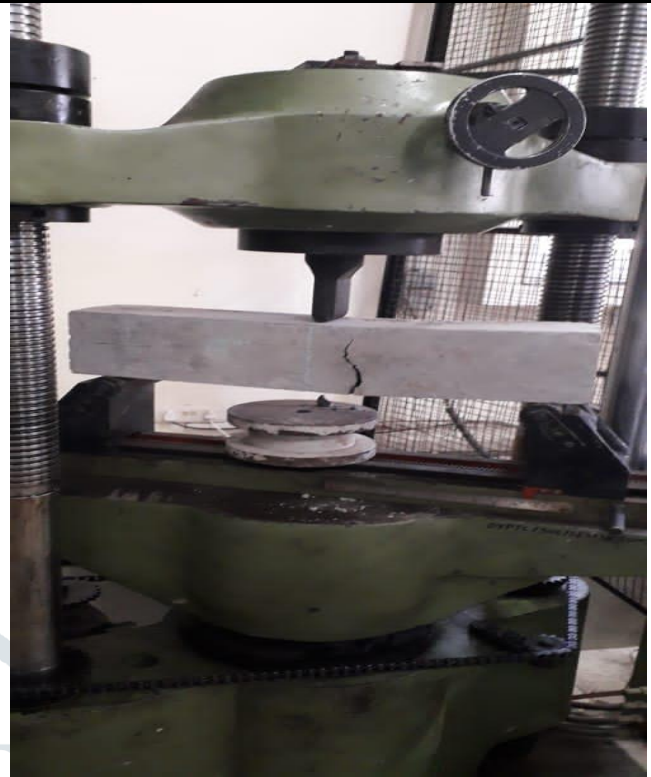
Fig. 2. Cracks developed in Bubble deck slabs.
