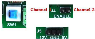
Figure 4.1(i) reset, supply pins, enable pins
