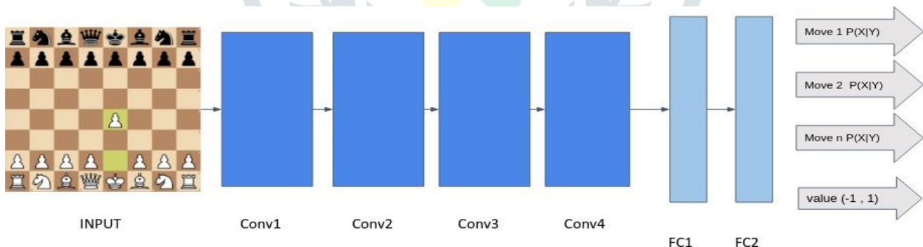
Fig 3. Visualization of move prediction network and neural network architecture
