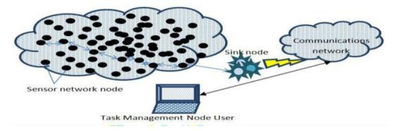
When transferring data, the sensor network is mostly dependent on distance, which is not a linear connection. The functional relationship is often an exponential function relationship, and it can be divided into a free space model and a multi-channel transmission model based on the distance. Figure depicts the wireless sensor network node model.
