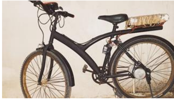
Fig. 1. PMDC motor connected to e - bike.
