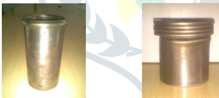
(a) (b) Fig 2. (a) Initial compression (b) Final compression
