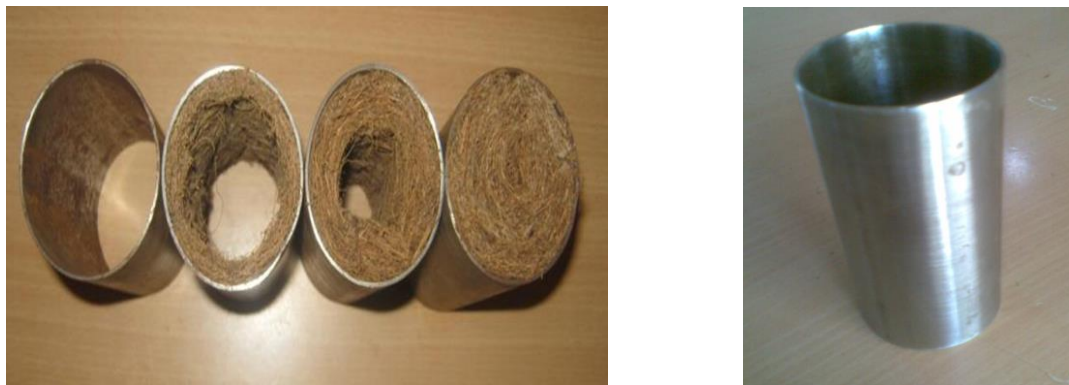
(a) (b) Fig. 1 (a) Difference in coir filling (b) Machined specimen
