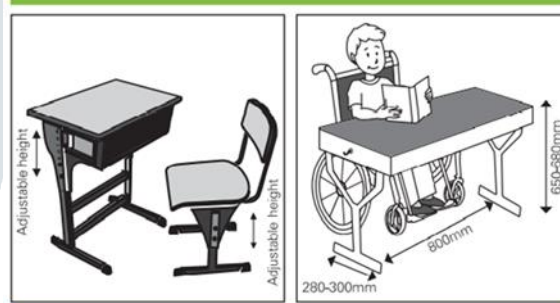
Figure 20: Detached desk and chair with height adjustable function Figure 21: Dimensions of accessible furniture
