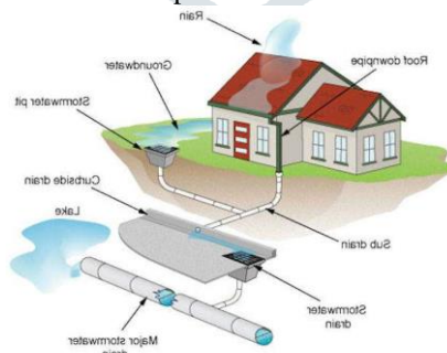
Fig 1. Storm sewer system
