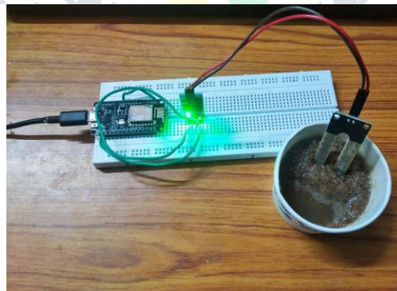
Fig 4: Soil moisture monitoring system set-up
