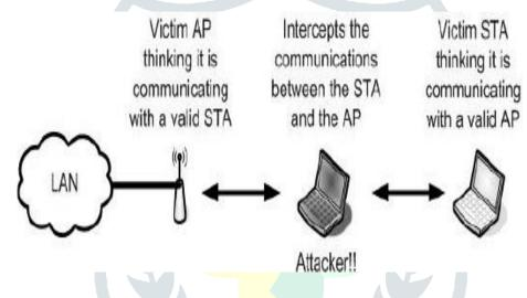
Figure 3: Representation of Man-in-Middle attack
