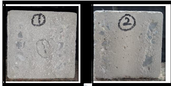
Fig. 2.12 Sample after Sand Blasting
