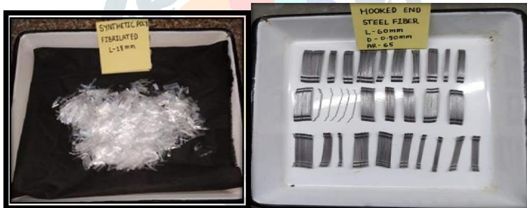
Fig. 2.2 Polypropylene and Steel Fiber
