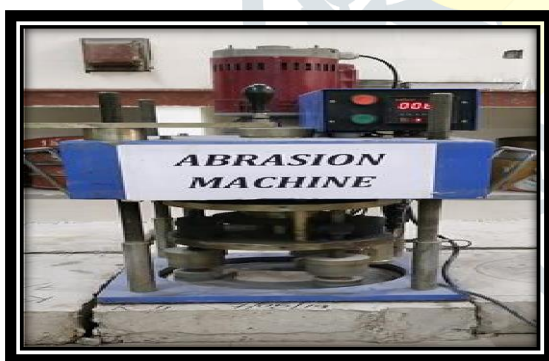
Fig. 2.8 Abrasion resistance test on concrete in slab
