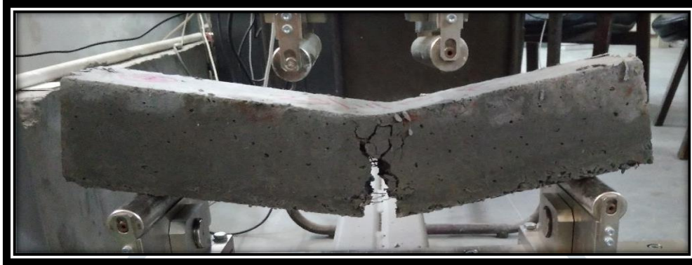
Fig. 2.6 Flexural strength test in progress
