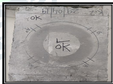
Fig. 2.9 Slab after abrasion test
