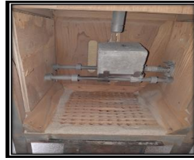
Fig. 2.11 Sample under Sand Blasting
