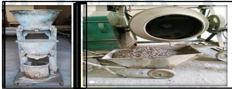
Fig. 2.3 Compacting Factor Apparatus
