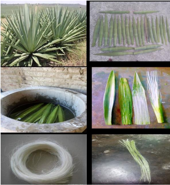
Fig 3.2 Sisal fiber extraction process
