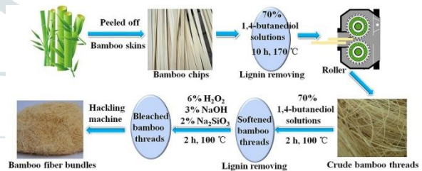
Fig 3.1 Bamboo fiber extraction process
