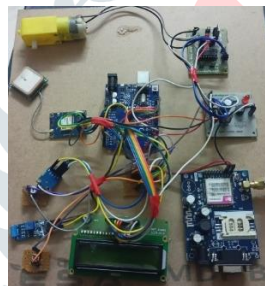
Fig.4: This is a prototype of the proposed system, which comprises sensors and other pieces of hardware equipment to detect an accident and to manage the vehicle's speed. A message will also be sent to the rescue crew, the hospital, or family members by the system.
