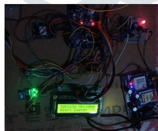
Fig.5: After the power supply has been connected, this is the Prototype of the system that is being suggested. It greets the user with the VEHICLE ACCIDENT ALERT SYSTEM displayed on the screen. Initially, sensors monitor the status of the device; if an accident happens, the gadget sends a message; otherwise, it continues functioning normally.
