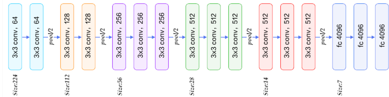
Figure 1. Basic VGG16 Architecture [18]
