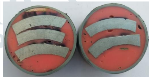
Fig.10. Al-Si alloy specimen prepared for the study of microstructure
