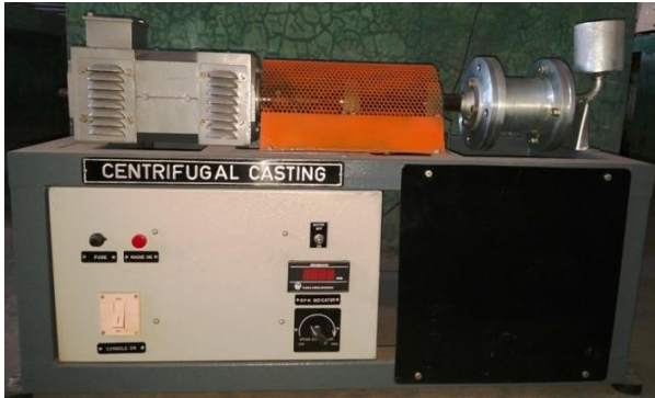
Fig.2. Centrifugal casting setup
