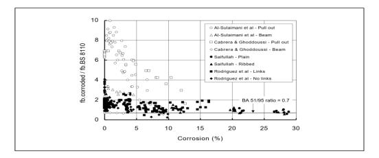
Chart-4 The effect of corrosion on the bond strength of reinforcing bars in comparison to the ultimate bond strength requirement of BS 8110
