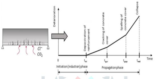
Fig1.2 Corrosion initiation and propagation times in reinforced concrete structures (Tuutti's model)
