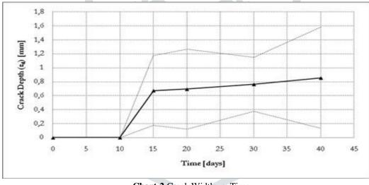
Chart-2 Crack Width vs. Time
