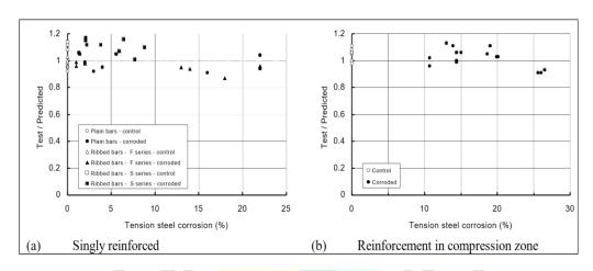
Chart-5 Corrosion affects the ratio of test/predicted flexural load-carrying capability for (a) those with compression zone reinforcement.
