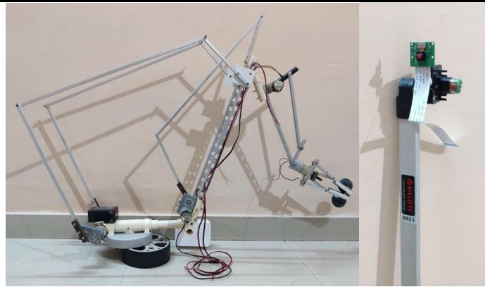
Fig 4.5 Fabricated model with concentric arm and camera and gripper is mounted with suction cups
