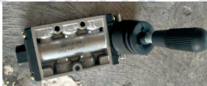
Fig no -6.5 -Position Control Valve
